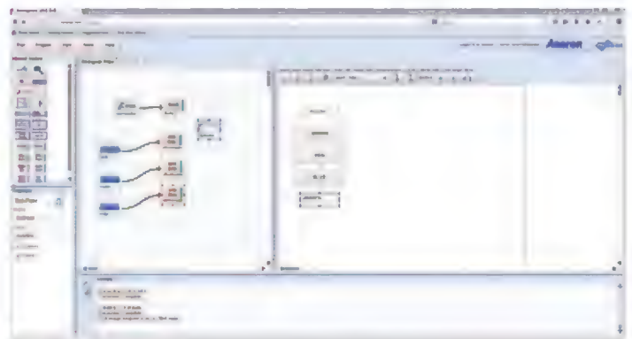
■ Screenshot 1. This is a view of the Atmosphere web window. The act of selecting objects from the Element Toolbox spawns behind-the-scenes graphics and code stub creation processes.
